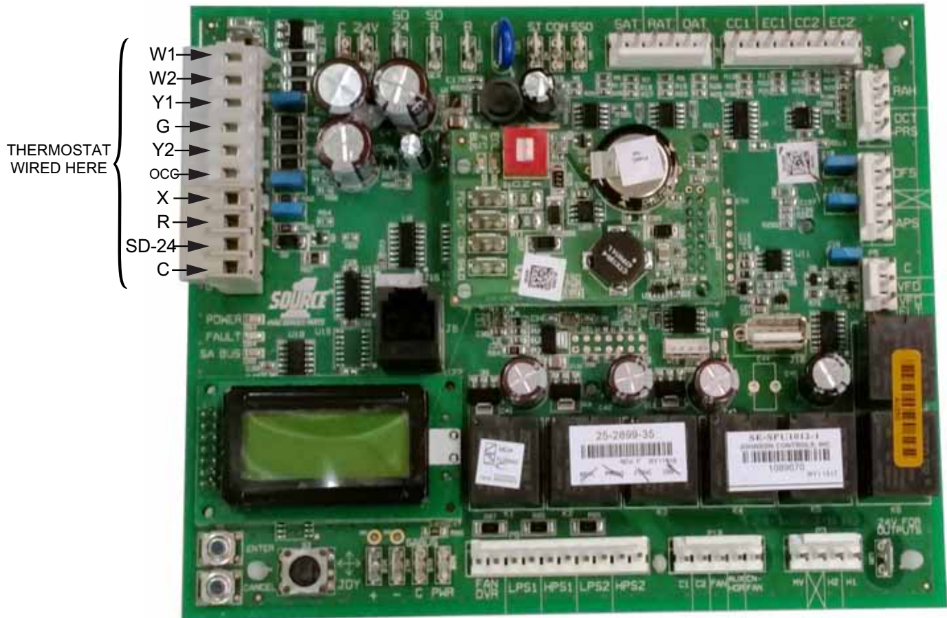
Figure 30: Unit Control Board
